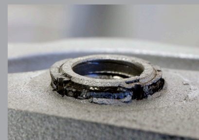
Original Failed Rocker Box Insert
